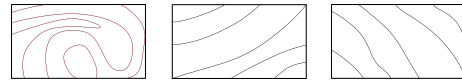
Figure 5. Epipolar lines. Left: not handled by our method; Middle and right: acceptable by our method.
