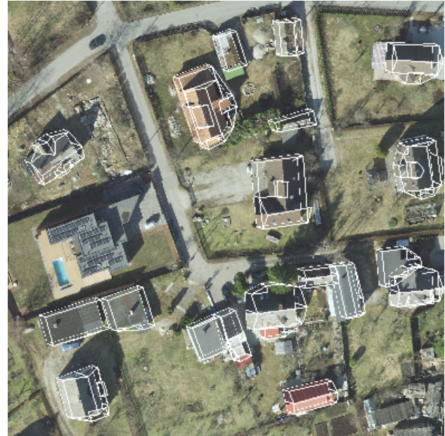
Figure 1. Example of LOD2-FORMER reconstruction on Talinn area. The background shows an aerial orthoimage of a residential block, while the overlaid white polygons depict LoD2 building wireframes. The figure illustrates that the model recovers complex multi-part roofs and ridges for detached houses and building blocks.
