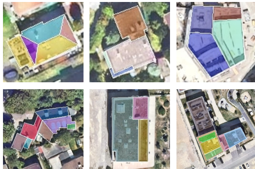
Figure 5. Manual labeling examples. The white lines indicate interpreted roof edges, while the different colors represent individual roof planes resulting from the manual labeling process.
