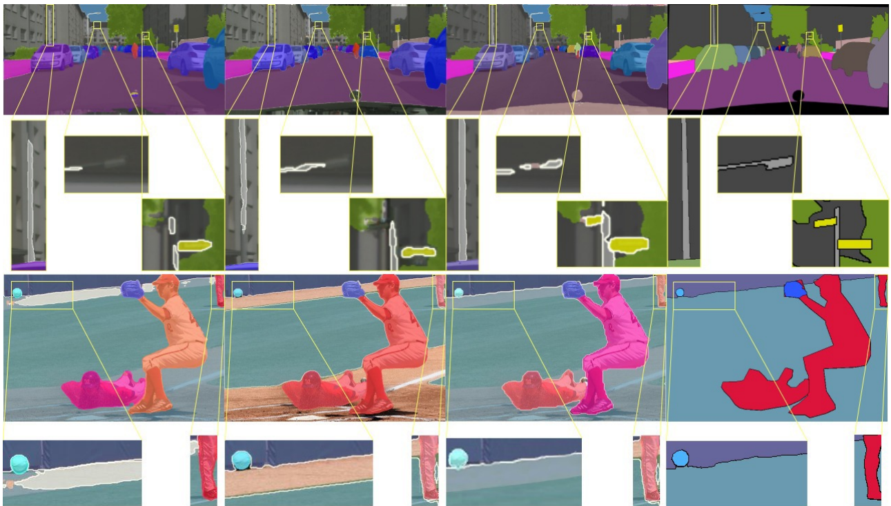
Figure 4. Comparison of CNN-, transformer- and Mamba-based architectures. From left to right: Panoptic-DeepLab (ResNet-50), Mask2Former(Swin-T), our model and finally the ground truth. The two examples are from Cityscapes and COCO, respectively.
