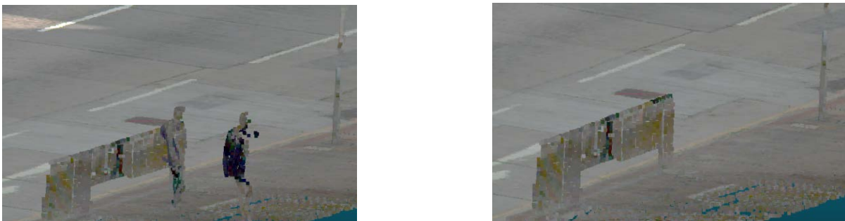
Figure 5. Comparison of pedestrian noise removal before and after processing
