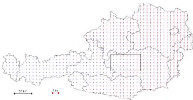
Figure 5. Height-Grid in Austria for transforming from orthometric to national MGI heights (overlaid with the test block boundary).
