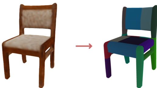
Figure 3. The CSDF rendered as a 3D texture (left) and the resulting convex decomposition (right).
