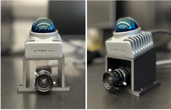
Figure 4. Custom handheld LiDAR-Camera scanner with hardware synchronization for data acquisition
