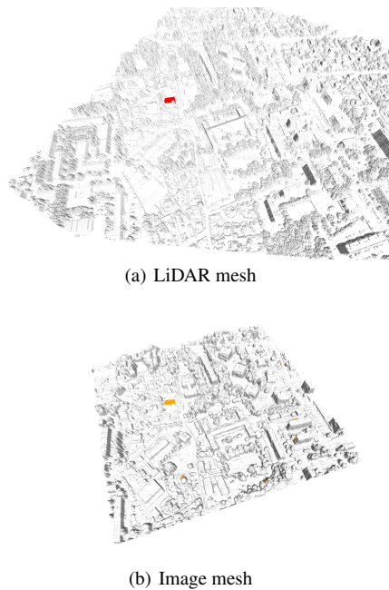
Figure 11. After removing small areas, most false alarms are eliminated. Red indicates inconsistent areas ③, and orange indicates inconsistent areas ④.
