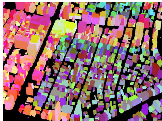
Figure 6. Projection image viewed by an oblique camera with the off-nadir angle of 45°
