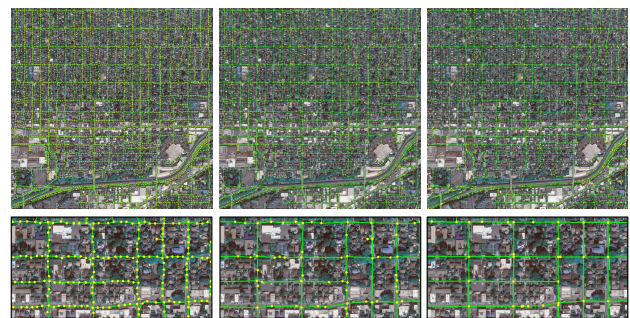
Figure 1. Our algorithm extracts road networks as low-complexity graphs while preserving geometric regularities (e.g., parallelism and orthogonality) and guaranteeing key applicability properties such as the graph planarity (right). In contrast, a state-of-the-art method such as SAM-Road (Hetang et al., 2024) produces an overly complex and irregular graph, prone to geometric defects (left). Simplifying SAM-road results with the popular Douglas-Peucker method reduces the complexity of the graph, but increases defects and irregularity (center).
