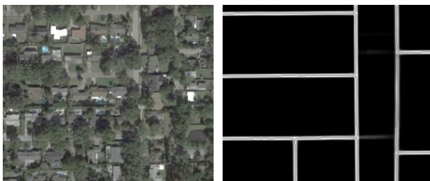
Figure 3. Centerline extraction. The centerlines (right, thin red lines on white pixels) are extracted as the one-pixel-thickness skeleton from the probability map. Note that centerlines are often wavy at some locations: this pixel-level noise is typically absorbed by the line-segment detector.
