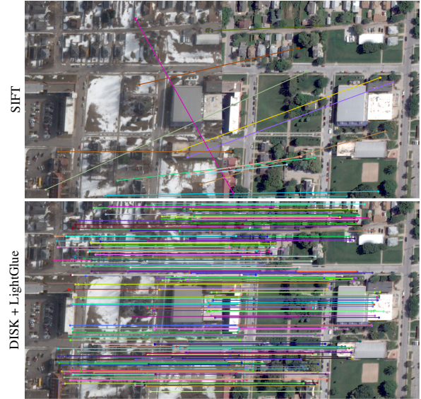
Figure 2. Comparison of SIFT and DISK+LightGlue matches for the diachronic pair OMA_331_017 – OMA_331_036.
