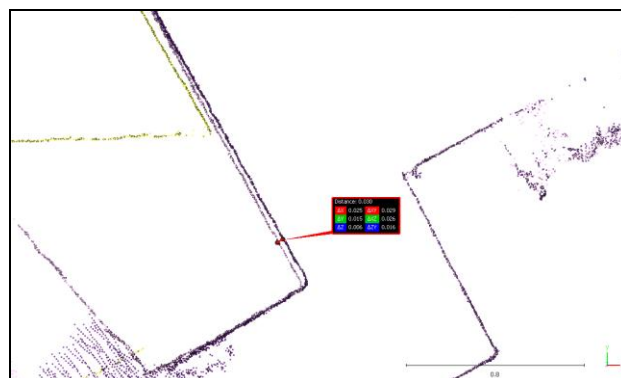
Figure 12. Cross-sections performed on the TLS and SLAM point clouds to verify the presence of any misalignments, evidencing a 3 cm discrepancy.
