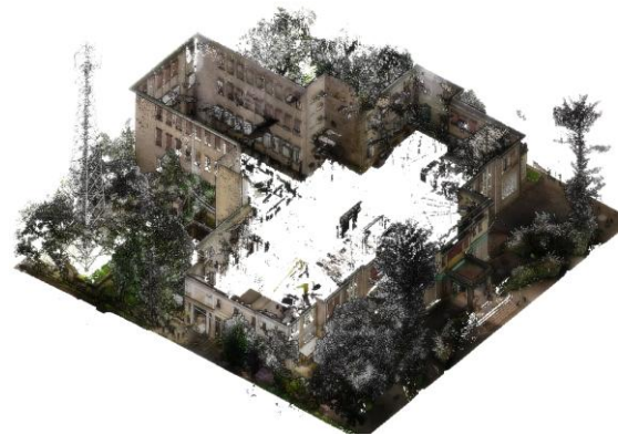
Figure 3. TLS point cloud after registration.
