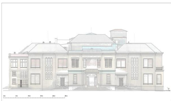
Figure 15. 2D drawing of main facade derived from Orthophotos generated from the TLS and UAV point cloud and vectorized in AutoCad
