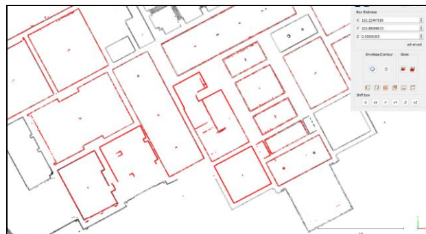
Figure 11. Cross-sections were generated from the TLS and SLAM point clouds to verify the absence of misalignments.
