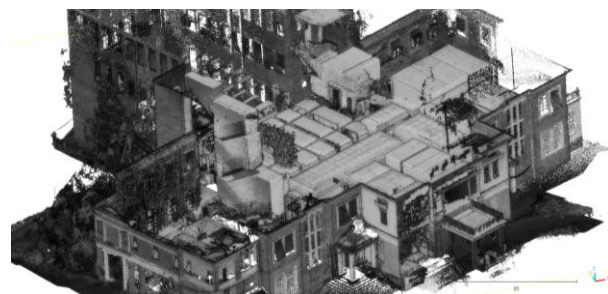
Figure 5. Outdoor and indoor mixed SLAM-based acquisition.
