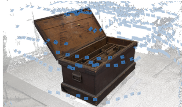
Figure 7. Photogrammetric mesh object trimmed from surrounding scene geometry
