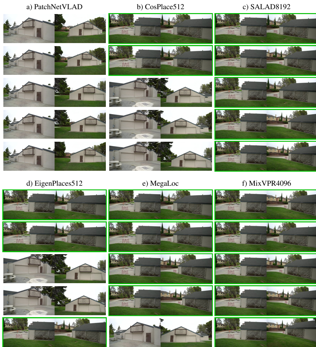
Figure 2. Qualitative top-5 retrieval results for different VPR methods on the T&T scene Barn . This scene is especially prone to perceptual aliasing, as indicated by the brown door, which is at different positions on both sides and the color of the floor in front of the house. Overlap areas are the back of the house, which is completely correctly retrieved by SALAD8192 and MixVPR4096. Columns correspond to methods (a–f) and, within each column, pairwise image matches are shown from rank k = 1 (top) to k = 5 (bottom) based on descending cosine similarity results. True positive matches are framed in green.
