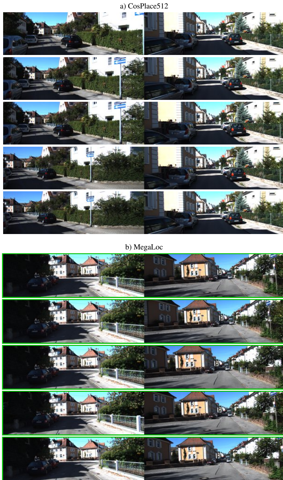
Figure 3. Qualitative Top-5 retrieval results from CosPlace512 (a) and MegaLoc (b) for KITTI scene 07_02. The challenge here is that some images were left out between A and B . This is especially important for tasks such as SLAM relocalization caused from missing frames. CosPlace (Berton et al., 2022) completely fails here, likely because of perceptual aliasing, indicated by two different black cars in A and B and other similarities, whereas MegaLoc (Berton and Masone, 2025) yields only true positives. The cue for correct results is the houses in the center of the A images, which appear towards the left border of the B images. Pairwise image matches are shown from rank k = 1 (top) to k = 5 (bottom) based on descending cosine similarity results. True positive matches are framed in green.
