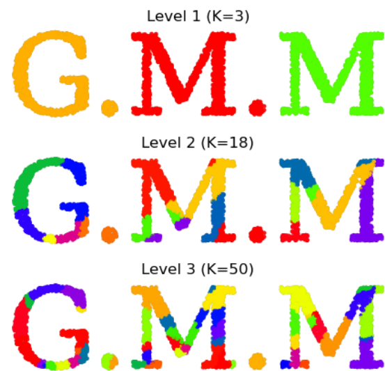
Figure 3. hGMM. Our method takes as input a point cloud and generates an initial segmentation (level 1) by fitting a coarse Gaussian Mixture Model (GMM) over the entire scene. Each resulting cluster is then refined through the estimation of a local GMM, leading to a hierarchical decomposition of the scene into increasingly fine-grained clusters (level 2 and level 3). The value K denotes the total number of Gaussian components at each level across all branches. Some components may remain empty when a region contains insufficient points, which accounts for the non-round progression ( K = 3 \rightarrow K = 18 \rightarrow K = 50 ).
