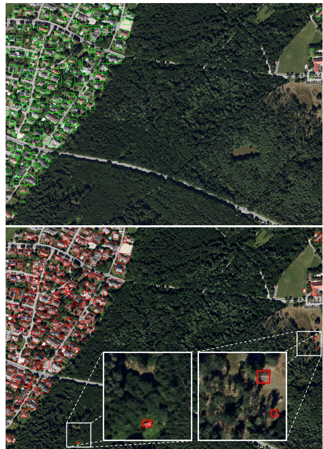
Figure 4. Comparison of the ground truth (above) and detected building footprints (below). Several small cabins in white rectangles are newly detected and absent from the BBD.
