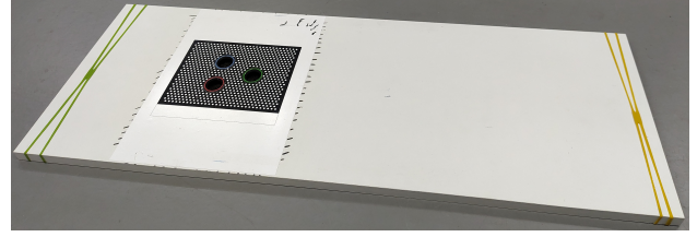
(a) In-house-designed wooden referencing plate demonstrator which is not sufficiently flat and can be deformed by the mobile robot weight. Green and yellow rubber band is applied against slipping.
