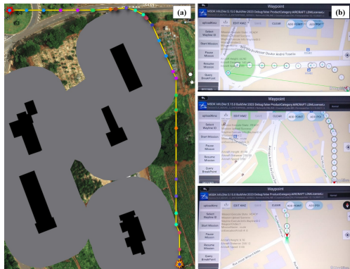
Figure 5. (a) Result of the route file creation stage in DJI WPML format, where each color corresponds to a new file. (b) Route execution using the DJI MSXK considering the same route files.
