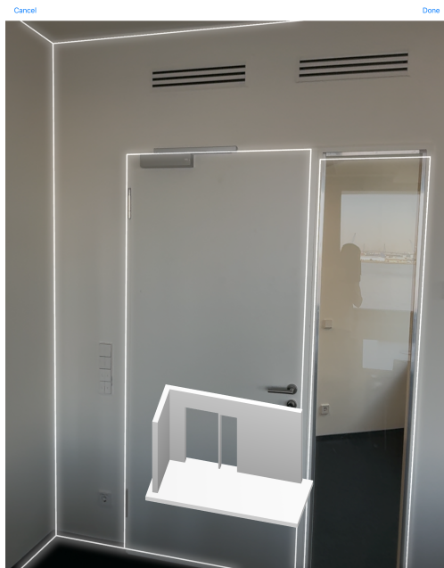
Figure 7. Exemplary office room captured in 3D using RoomPlan API. Windows, doors, floor and walls are detected and reconstructed in a local coordinate reference system.
