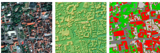
Figure 4. Detail section of test region Memmingen, 500 \times 500 m 2 , left: True ortho image from the Pléiades-scene, center: DSM, right: derived classification (blue: water, light-green: grass, dark-green: tree, red: adobe roof tiles, light-gray: concrete on flat roofs, dark-gray: asphalt/road, yellow: bare soil).
