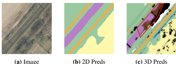
Figure 5. Comparison of 2D and 3D predictions, where incorrect 3D predictions can override correct 2D results when fused, potentially indicating false changes.
