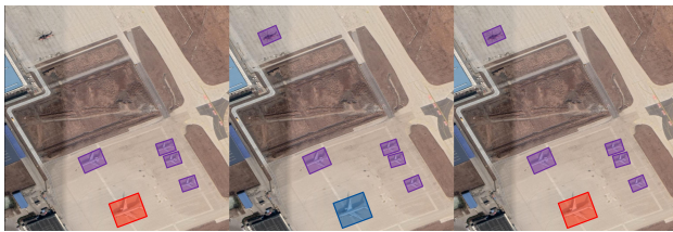
Figure 7. Example results of practical experiments: Classification results of the baseline model (center) have been updated (right) with given priors and proved by GT labels (left). The misclassification from A350 (red) to B747 (blue) has been corrected. One Helicopter (top left of the scene) has been additionally detected and labeled as “other” (purple).
