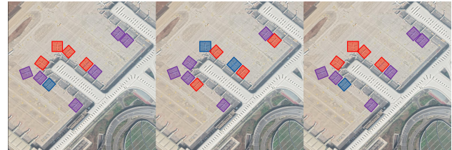
Figure 6. Example results of oracle experiment: Classification results of the baseline model (center) have been updated (right) with given priors and proved by GT labels (left). The misclassification of B737 (red), A220 (purple), and “other” (blue) has been corrected.
