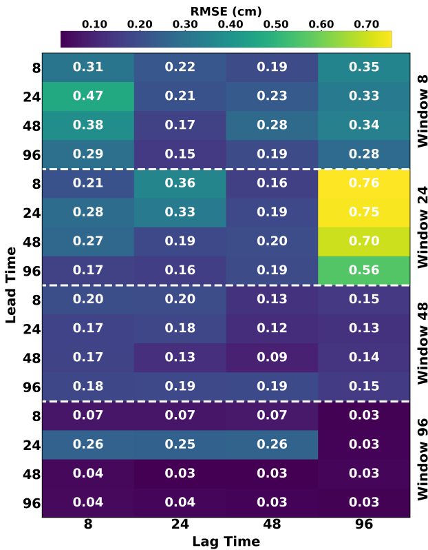
Figure 3. RMSE values of sea ice thickness prediction using various lag, lead and window sizes.
