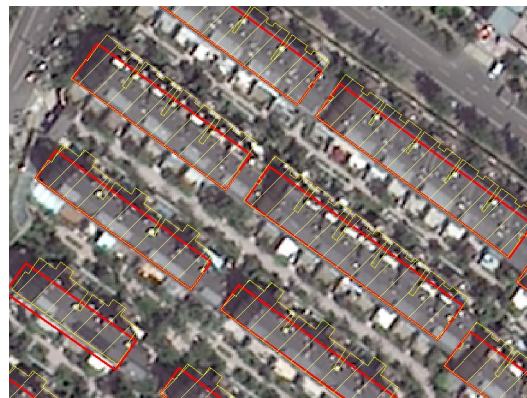
Figure 5. Type 2: difference between house examples in NFSM and UTSM (the red is UTSM and the yellow grid is NFSM)
