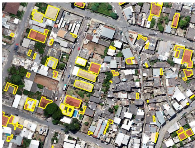
Figure 2. Example of ceramic rooftop labeling, illustrating the variation in building patterns observed throughout the study area.
