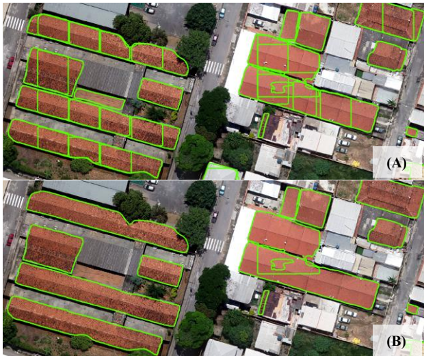
Figure 4. Topological adjustment of generated segments. (A) Segmentation produced by the model. (B) Output after applying topological correction.
