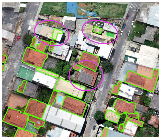
Figure 3. Rooftops predicted by the model. Lilac circles highlight light-colored or elongated rooftops that the model did not identify.
