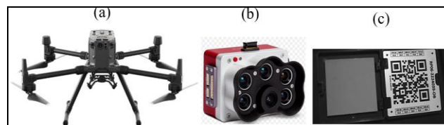
Figure 2. The instruments employed for UAV multispectral imagery acquisition were: (a) DJI Matrice 300 UAV, (b) Micasense RedEdge-P camera, and (c) MicaSense Calibrated Reflectance Panel..
