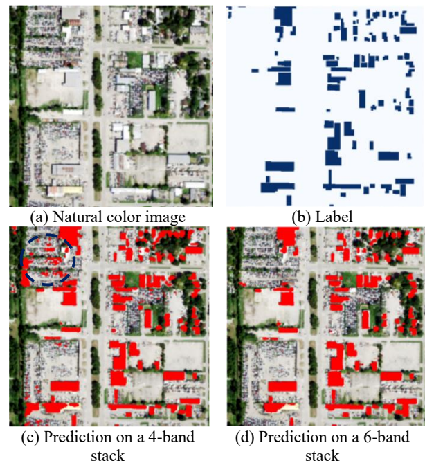
Figure 3. An example of building footprint extraction results on the data. Columns (from left to right) show the RGB image (a), ground truth building mask (b), and prediction overlay on the RGB image for 4-band (c) and 6-band (d) respectively. National Agriculture Imagery Program imagery accessed via the U.S. Geological Survey EarthExplorer portal.
