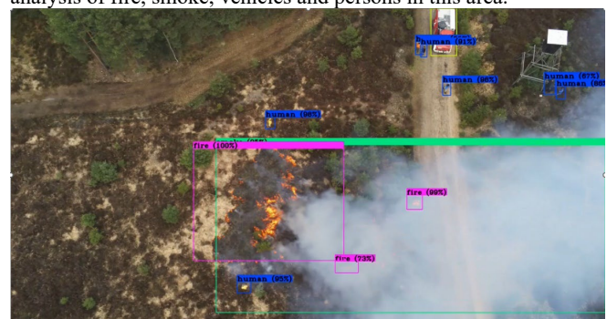
Figure 19. AI based assistance for the fire brigade to monitor and assist in the defence
