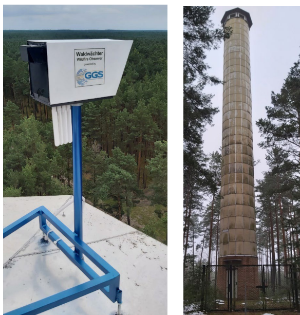
Figure 10. Fireguard360 Camera gimbal on the Tower Podrosche left and the tower itself
