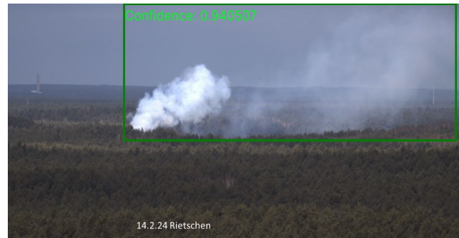
Figure 11. AI based detection of a smoke bomb test from Firewatchtower Rietschen
