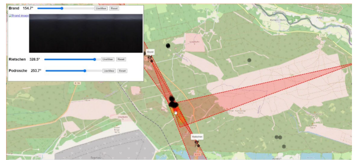
Figure 15. Triangulation to determining the fire hotspot
