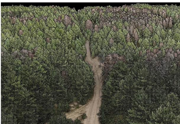
Image 7. Very dense Point-cloud generated with DJI Matrice 350 and L2 LiDAR of the test-plot
