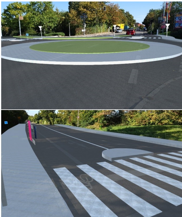
Figure 5. Situated AR demonstrator showing aligned planning models in an outdoor environment.
