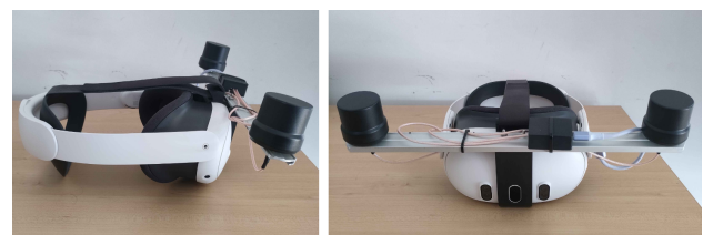
Figure 3. Prototype: 2 antennas connected to a Unicore UM982, with a 30cm baseline, and attached to a Quest 3 XR headset.
