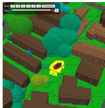
Figure 4. Demonstration of fire simulation on Hologram Table at UNSW MERE. The voxel colors represent fire spread states (red: burning, yellow: heating) as well as corresponding fuel types, while the wind directions are illustrated by blue arrows.
