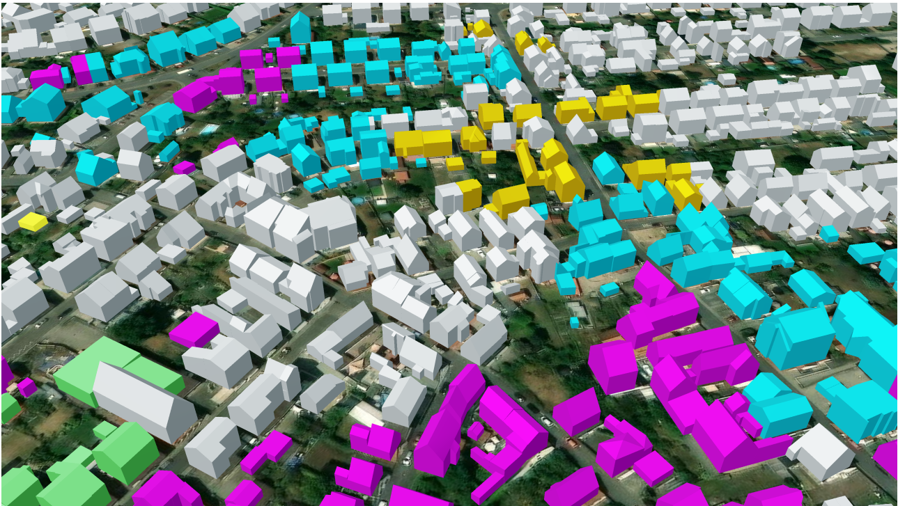
Figure 1. Visualization of buildings with enriched storey information in an excerpt of the test area of Heidelberg, Germany. For available Mapillary images, according building models are color-coded by number of floors based on our estimation: two (cyan), three (magenta), four (yellow), five (green), or none (gray). Visualized using CesiumJS and 3DCityDB Web Map Client, with ArcGIS World Imagery as the basemap.
