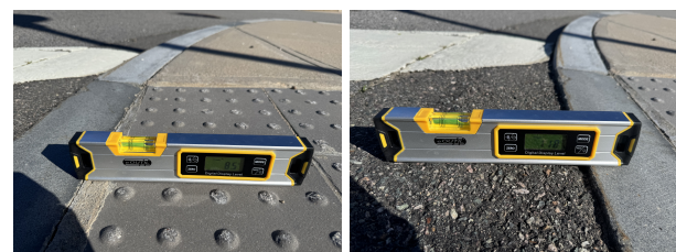
Figure 8. Slope validation process using a physical 12-inch (0.3048 m) inclinometer. Using the inclinometer, we inspect intra-feature slope (left) and inter-feature slope (right) for selected sidewalk features in our point of interest.
