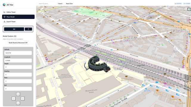
Figure 7. Screenshot of 3DTiler web app, georeferencing a building model on the UoC Campus.
