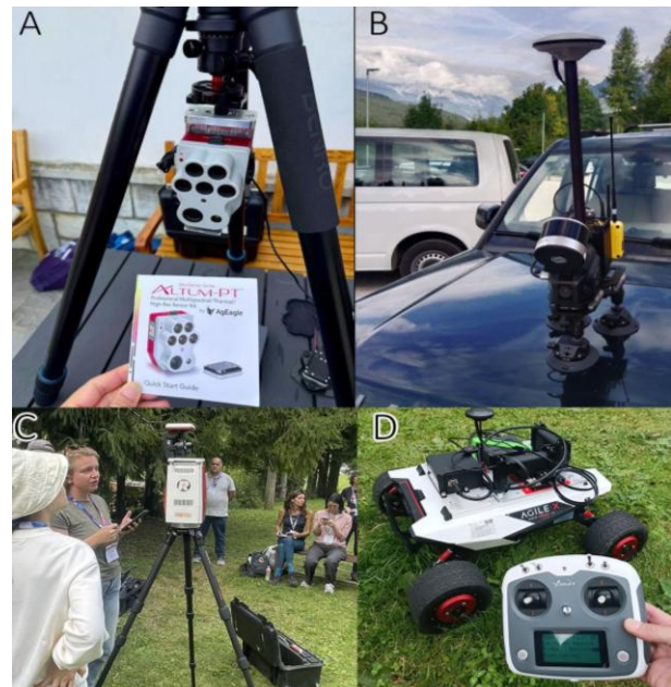
Figure 2. MicaSense Altum PT (A), Stonex x120go SLAM (B), Riegl VZ600-i (C) and SILVA Rover by CISAS (D).
