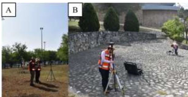
Figure 2. Equipment used in the field: (A) RTK positioning system, (B) RTK positioning system and DJI Matrice 350 with the Zenmuse L2 sensor.
