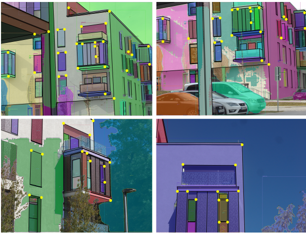
Figure 9. SIOCP matching points with instance-segmented façade elements and their matched edges in the background.
