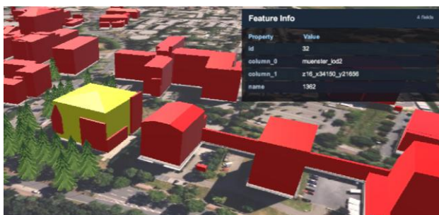
Figure 11. Metadata retrieval using raycasting hit point and PostGIS 3D querying
