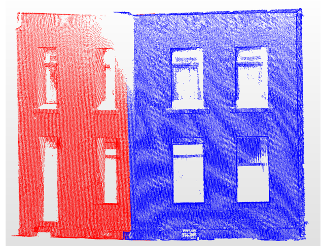
Figure 3. Facade isolation and plane segmentation in the LiDAR workflow, with each colour representing a distinct RANSAC fitted wall plane.
