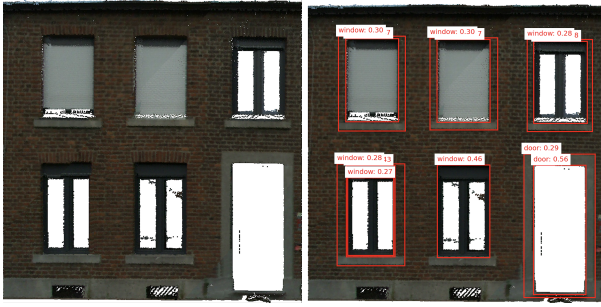
Figure 4. Facade projection and opening detection. Left: RGB raster image from MLS facade points projected onto the RANSAC fitted plane. Right: Raw Grounding DINO detections with confidence scores, before postprocessing.
