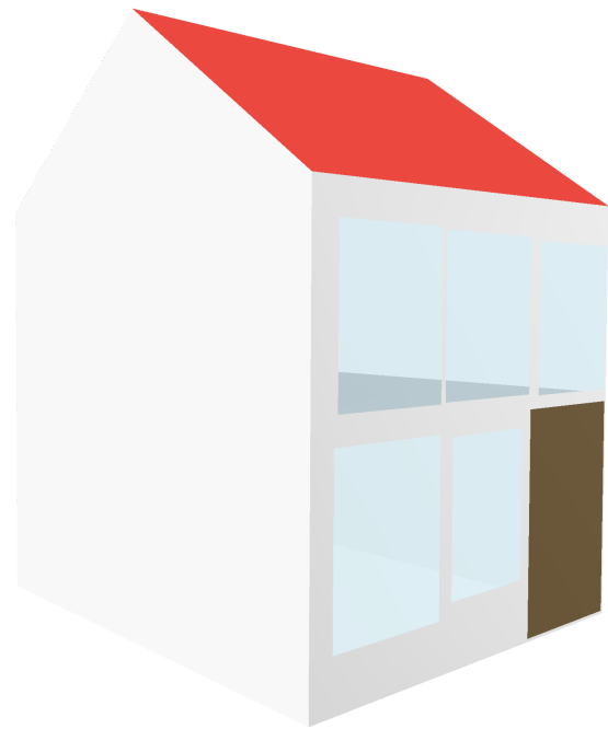
Figure 7. Enriched LoD3 CityJSON building model with Window (light blue), Door (brown), FloorSurface, and RoofSurface (red) semantics.
