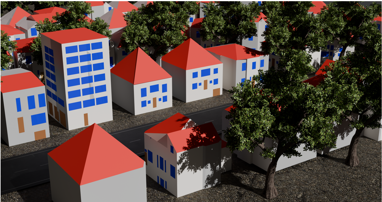
Figure 1. Reconstructed façade openings for LoD3 building models in a selected exemplary neighborhood in Hamburg, Germany, visualized in Blender ® . Blue rectangles indicate reconstructed windows, while brown rectangles indicate reconstructed doors.
