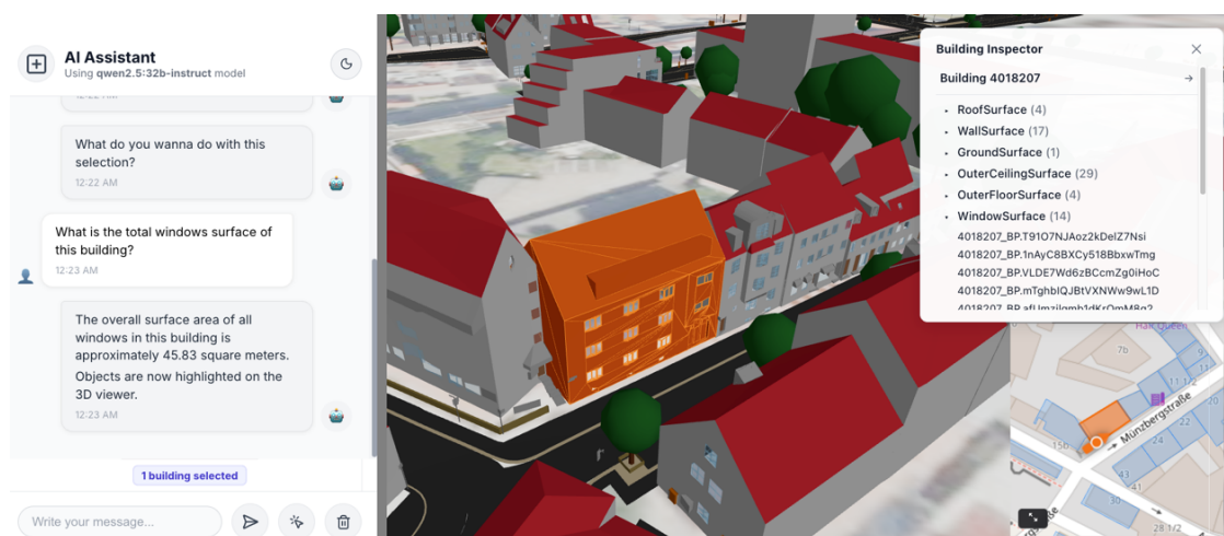
Figure 5. Interaction with the LLM agent and a Threejs based 3D Viewer using the MCP Server
