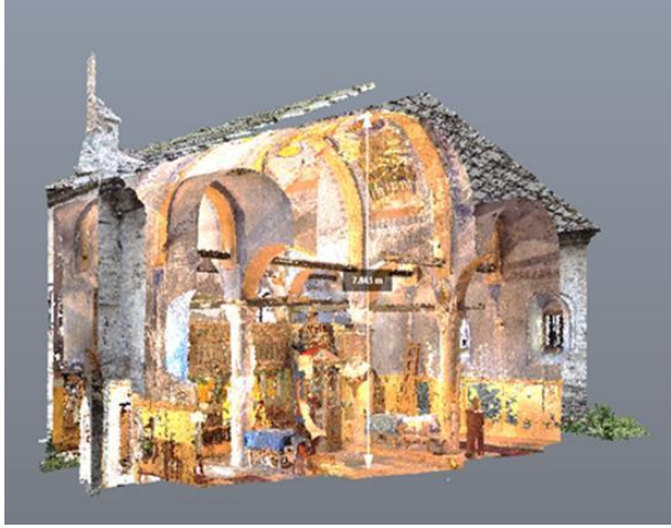
Figure 5. Approximate interior height of the Church of St. Petka relevant for photogrammetric image acquisition.
