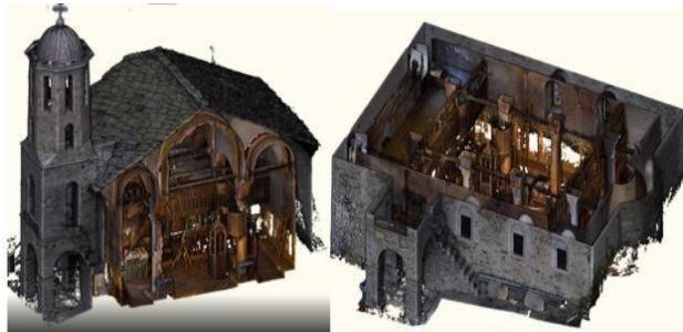
Figure 8. Point cloud obtained from UAV-based close-range photogrammetry.
