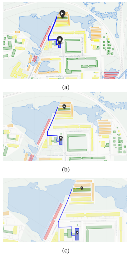
Figure 5. Local-scale example of route behaviour in Case 5. Sub-figures (a)–(c) show progressively closer views of the affected area. The flooded segment is excluded from routing, while the remaining dry segments preserve route connectivity.
