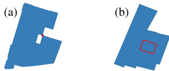
Figure 3. Geometric errors in the input data. (a) Self-intersection; (b) Nested inner rings.
