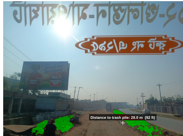
Figure 6. Representative Mapillary image captured from an in-vehicle perspective, along with the corresponding roadside waste segmentation and successfully predicted depth with respect to the camera's GPS coordinates.
